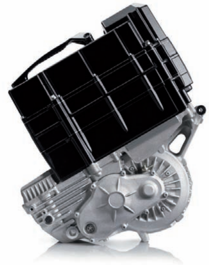
Figure 1: With up to 30 HP and 42 Newton meters from the HEINZMANN disc motor the Freeride E is equivalent to a 125.
